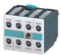
Auxiliary switch block, 22, 2 NO + 2 NC, EN 50012, 4-pole, screw terminal, for motor contactors, Size S0 .. S3 ! Phased-out product! Successor is SIRIUS 3RH2
