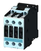
Power contactor, AC-3 9 A, 4 kW / 400 V 230 V AC, 50 Hz, 3-pole Size S0 Screw terminal !!! Phased-out product !!! Successor is SIRIUS 3RT2 Preferred successor type is >>3RT2023-1AP00<<
